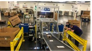
The small delivery unit sorter machine can sort at least 2,250 pieces an hour and requires less than 1,500 square feet of space.
